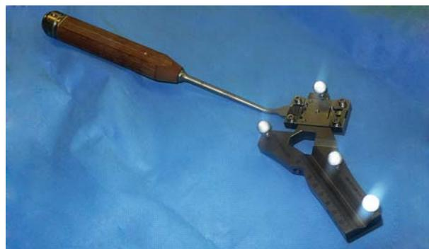
Navigated PAO chisel with calibration device.
