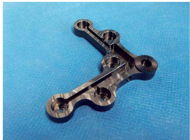
High accuracy tracking markers, constructed from titanium, allow measurement and control of a robotic system for minimally invasive cochlear implantation.
